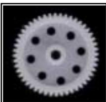
I used the gear driven by the motor pinion as my disk wheel. Each of the large gears in the box has 48 teeth, and each is meshed with a 12-toothed pinion dropping the motor speed by a factor of 4 in three stages. This means that the road wheel
