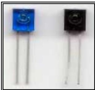
'side-looking' devices in a convenient square package easily stuck to the sides of the gearbox with impact adhesive. Looking at the picture of the assembled gearbox you can just see the tops of the LED and phototransistor fixed either side so as to 'look through' the holes in the gear as they go past. The circuit is quite
